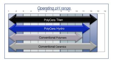
PolyCera Hydro membranes are made by a patented process of blending PolyCera and commodity polymers, which gives rise to membranes that exhibit robustness of the commodity polymer, but with unrivaled fouling tolerance and ease of cleaning.
