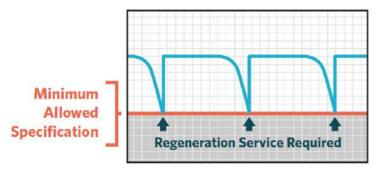
As ion-exchange resins exhaust, contaminants begin to break through, eventually requiring downtime for resin regeneration or replacement.
